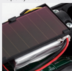
COMBINED OPERATION BATTERY - SOLAR PANEL
