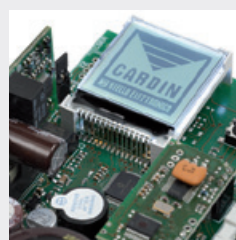
SELF-PROGRAMMING MONITORED BY AN LCD GRAPHICS DISPLAY
