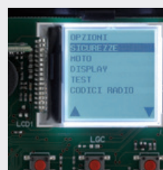
SELF-PROGRAMMING MONITORED BY AN LCD GRAPHICS DISPLAY ELDOM34
