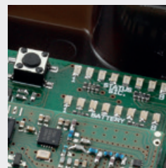
8 RED SAFETY STATUS LEDS 8 GREEN BATTERY CHARGE LEDS
