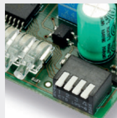
SENSITIVITY SELECTION DIP-SWITCHES
