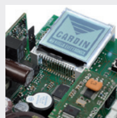
SELF-PROGRAMMING MONITORED BY AN LCD GRAPHICS DISPLAY
