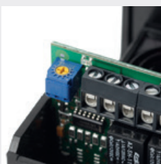
SENSITIVITY ADJUSTMENT TRIMMER
