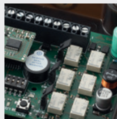
STATIONARY TRANSCEIVER, SAFETY OUTPUT MANAGEMENT (NC/8,2kΩ)
