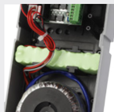
BATTERY CHARGER AND NiMH BATTERIES
