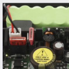
EMERGENCY NIMHBATTERIES IN THE CC242ETOPCB AND CC242EXTOPCB VERSIONS
