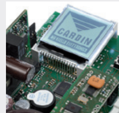
SELF-PROGRAMMING MONITORED BY AN LCD GRAPHICS DISPLAY
