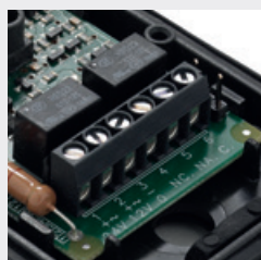
EXCHANGE CONTACT NC-NO-C
