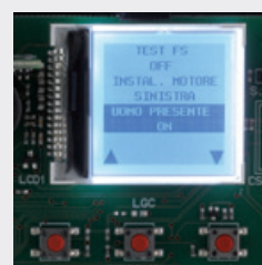
SELF-PROGRAMMING MONITORED BY AN LCD GRAPHICS DISPLAY CC242ETOP AND CC242EXTOPCB
