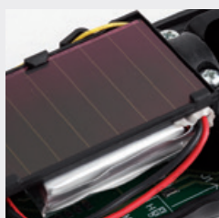
COMBINED OPERATION BATTERY - SOLAR PANEL ON THE PROJECTOR
