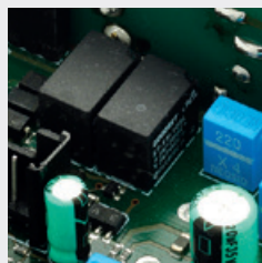
DOUBLE RELAY WITH SERIAL EXCHANGE NO-NC
